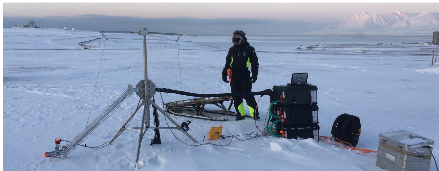
Measuring the stable isotope composition of the lower 2 m above snow, sea ice and open water at Ny Ålesund in February 2020 (photo: Harald Sodemann).
