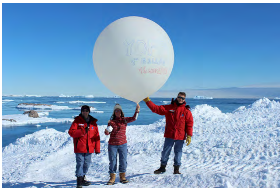
Radiosonde launch during first Antarctic summer Special Observing Period at French Antarctic station Dumont d'Urville (photo: Météo France).
