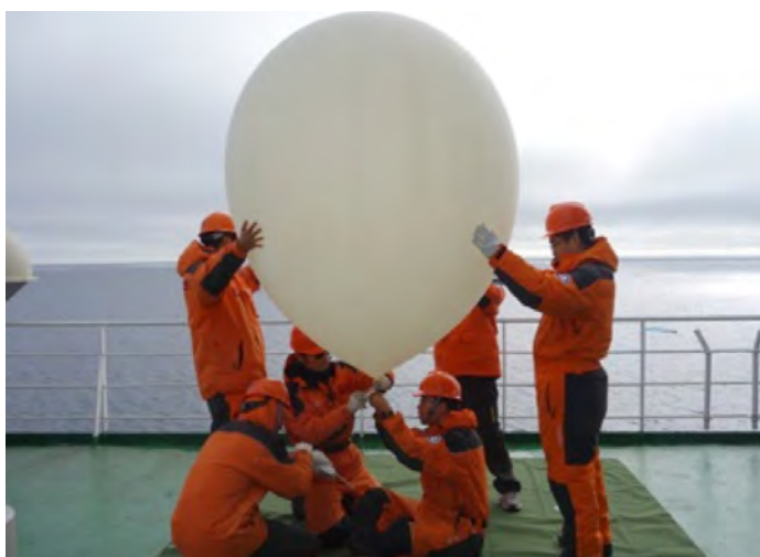
Expedition members are preparing the weather balloon aboard the Chinese icebreaker Xuelong before launching a radiosonde over the Arctic Ocean (photo: Dongqi Zhang/China Meteorological Administration).
