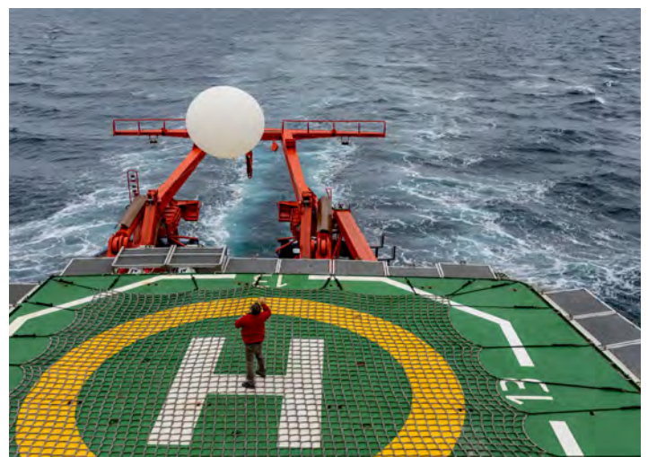
Radiosonde launch from the helicopter deck aboard RV Polarstern during SOP2 (photo: Christian Rohleder/DWD).
