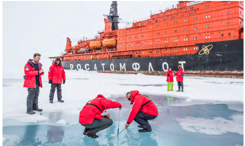
Participants of the cruise to the North Pole are measuring melt pond depth and salinity in the citizen-science project SIRT (photo: Lauren Farmer).
