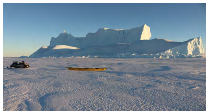
Kayak with the electromagnetic measuring device EM31 pulled across Atka Bay to determine snow and ice thickness (Photo: Stefanie Arndt/Alfred Wegener Institute).
