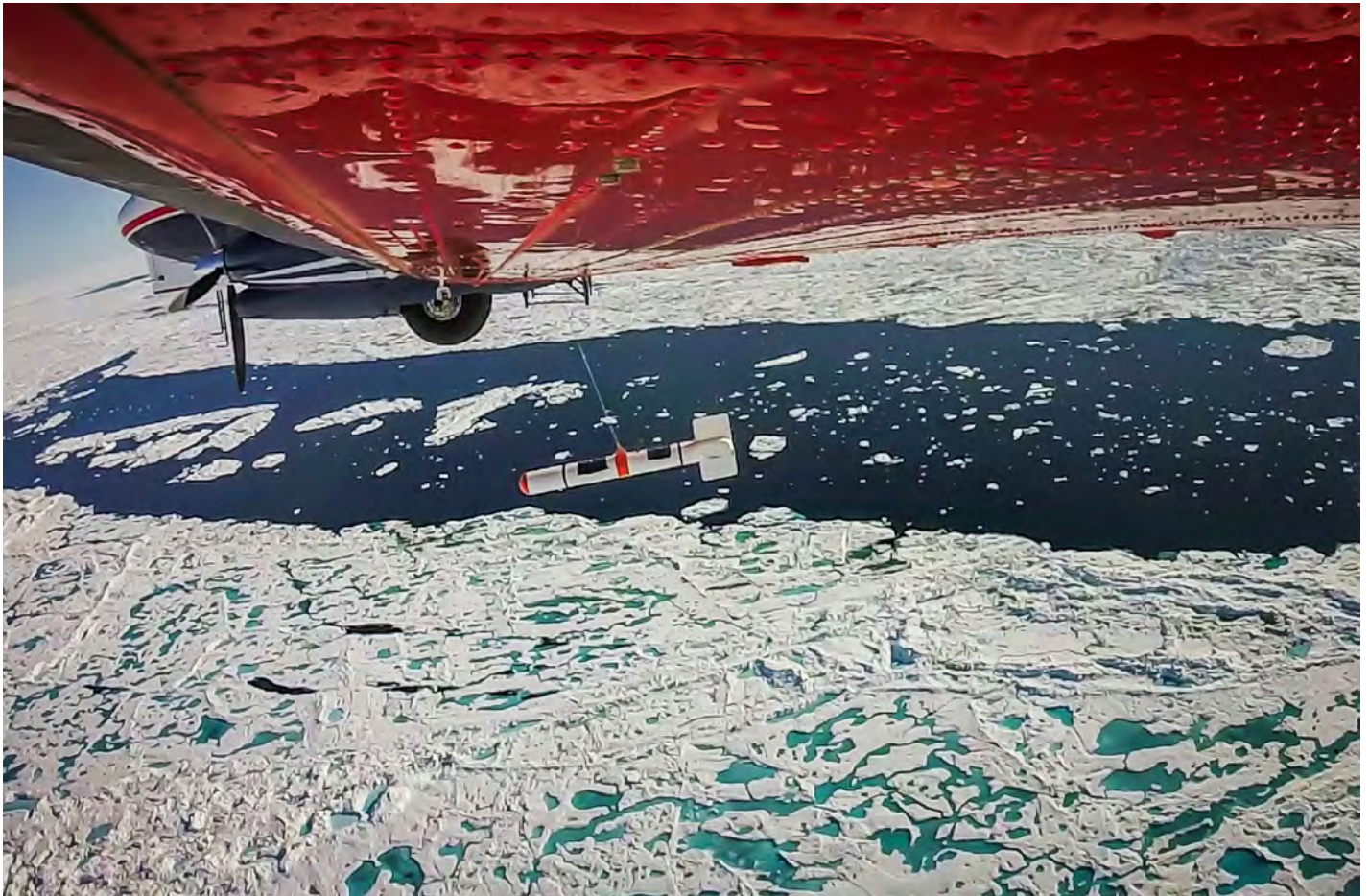
Low-level flight with Polar-6 aircraft over Northern Greenland sea-ice cover. Attached to the aircraft is the electromagnetic (EM) bird device to measure ice thickness (photo: Esther Horvath/Alfred Wegener Institute).
